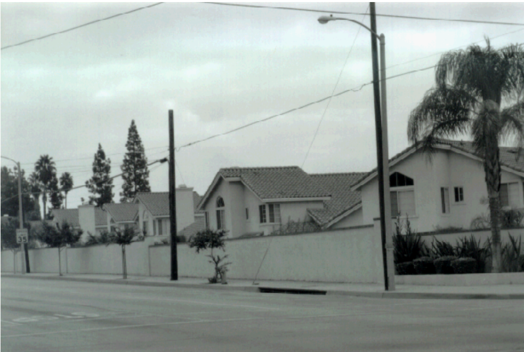
PICTURE 8. NEWER SINGLE-FAMILY DETACHED RESIDENTIAL DEVELOPMENT, AT SUNFLOWER AVENUE AND COVINA BOULEVARD. AN EXAMPLE OF AN APPROPRIATE NOISE-INHIBITING DESIGN STANDARD COMMONLY INCORPORATED INTO RESIDENTIAL PROJECTS ON MAJOR STREETS, DECORATIVE BLOCK WALLS SERVE AN IMPORTANT PURPOSE, AND, THEREFORE, THE GENERAL PLAN ADVOCATES THE CONTINUED USE OF THIS AND SIMILAR DESIGN FEATURES.
