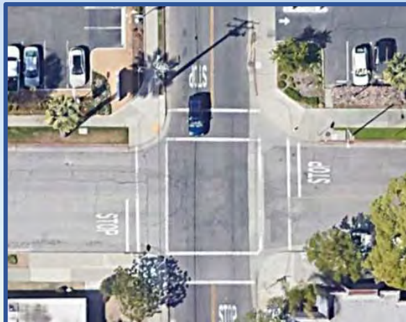
College Street/3 rd Avenue All-way stop control with standard crosswalk striping
