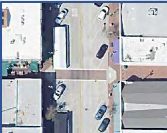
Midblock on Citrus Avenue Decorative uncontrolled midblock crosswalk near downtown
