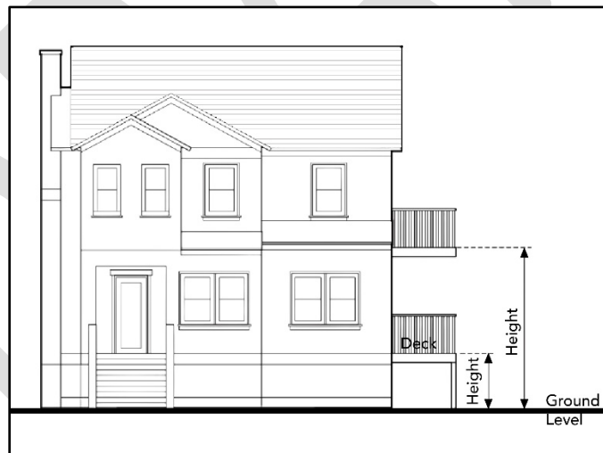
Figure 17.22-L Measuring Height of Decks
